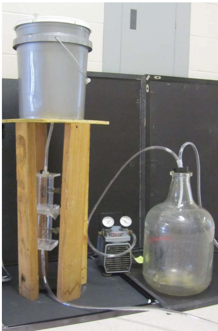
Figure 4.5: Closed System Filtration Apparatus with Mixer and Vacuum Pump
