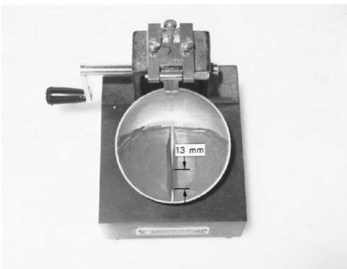
FIG. 8 Soil Pat After Groove Has Closed
